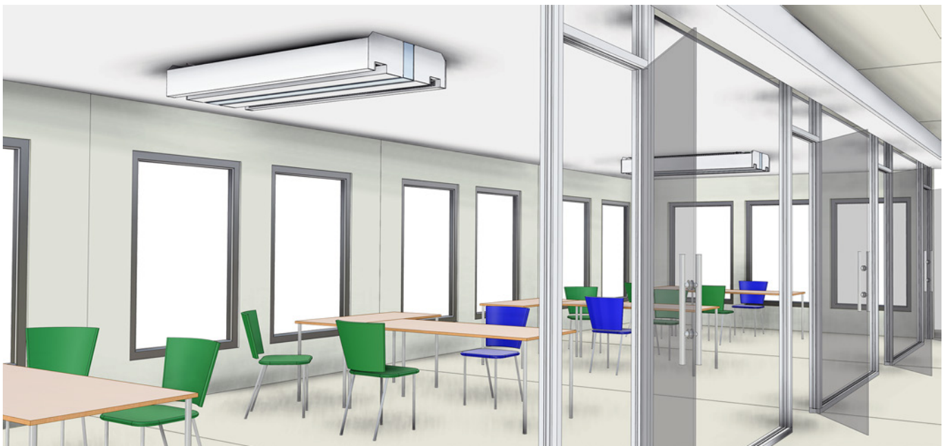
Picture 53. The partitions have been removed without affecting the Plafond installations.
